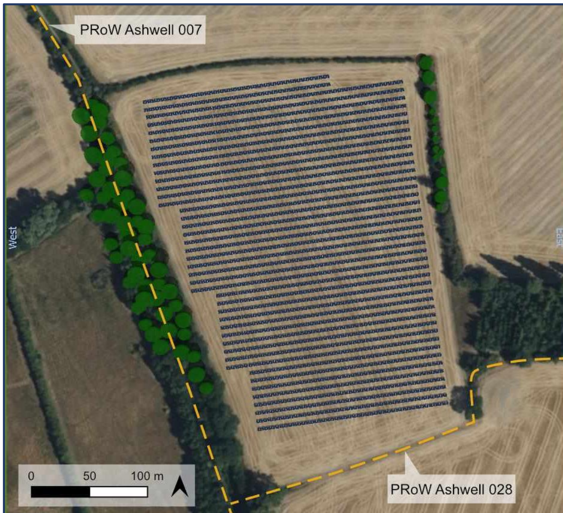
Figure 4.6 – Indicative Ground-Mounted PV layout at Love Lane, Ashwell.
