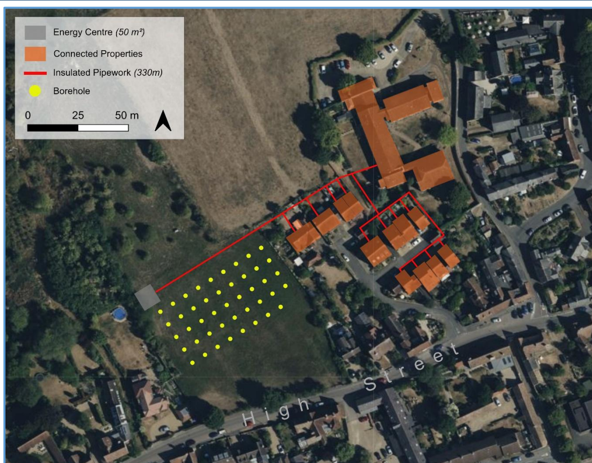
Figure 4.8 – Indicative Closed-Loop GSHP DHN Layout at Dixies Meadow, Ashwell.
